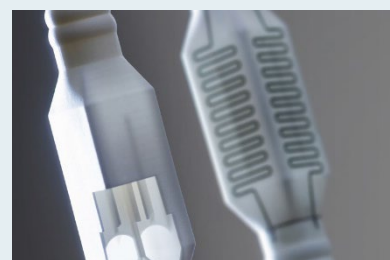
Figure 1: Print job preparation of a three-chamber fluid mixer (left), 3D-printed three-chamber fluid mixer with different wall thicknesses and hidden channels (center), additively manufactured fluid heater with printed conductors (right).
