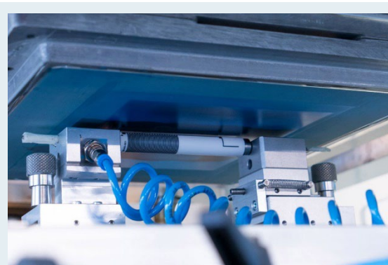
Figure 8: Circular screen printing for functionalization of tubular structures for heaters or flow sensors.
