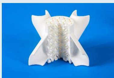
Figure 1: Print job preparation of a three-chamber fluid mixer (left), 3D-printed three-chamber fluid mixer with different wall thicknesses and hidden channels (center), additively manufactured fluid heater with printed conductors (right).
